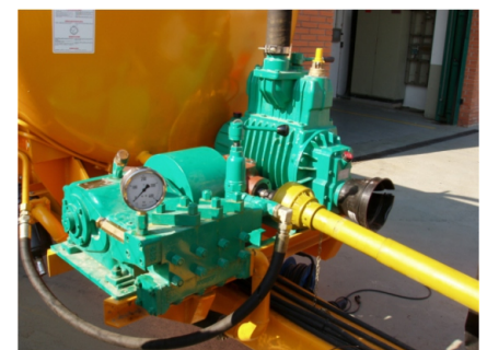
345A Driven by P.T.O. tractor 140 bar - 135 l/min
